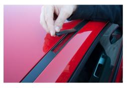
This will release the cover, lift 45 degrees up and slide out of the housing.
