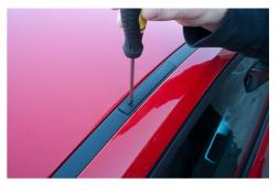
Use the 'flat head' screwdriver and turn the plastic cover screw 90 degrees.
