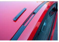
Each of the four channels are filled with a form of 'putty', the fix point is located in the centre of the channel.
