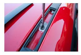
This will only unscrew to a point Using your fingers remove the screw.
