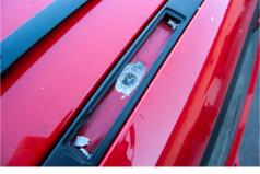
Once you have removed the covering layer of putty you will discover the plastic fix point retaining screw.
