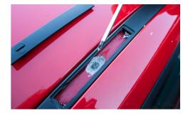
Using your 'philips head' screwdriver, remove the plastic retaining screw.
