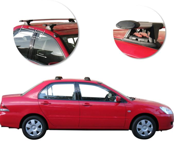
Roof rack: S16 Fitting Kit: K332 Max roof rack loading: 50 kgs Type of Fitment: Fixed Point Mount Available crossbar length: 1200mm Comments:
