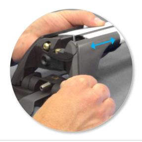
Adjust the legs on the crossbar to that they are positioned equally from the ends of the crossbar, and the clamps engage firmly on the body clip installed on the vehicle.
