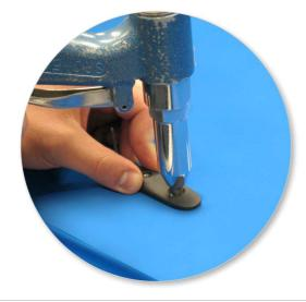
• While holding the permanent mount block firmly on roof, rivet the blocks to the roof.
