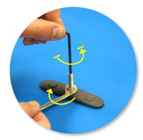
Using spanner supplied with crossbar and 3mm (1/8") Hex Key, back grubscrew off half a turn and lock nut down.
