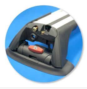
• Ensure the red plastic knob is in the position shown when fully tightened.
