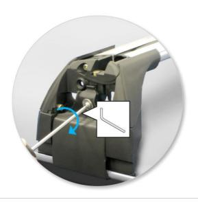
Use same capscrew and washer to secure clamp onto leg.
