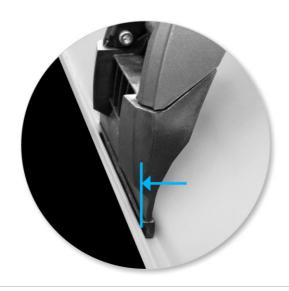
Loosely position crossbar ensuring the guttermount blade is hard against the inside of the vehicle gutter.
