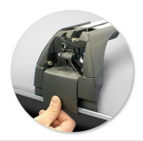
• Loosely line up clamp over the vehicle gutter.
