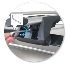
• Use 5mm Hex Key to tighten clamp and secure crossbar to rail.
