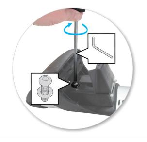
Using short capscrew and washer, secure assembly onto leg (use Hex Screwdriver supplied with crossbar to assist)
