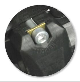
• Bolt should sit in groove as shown.
