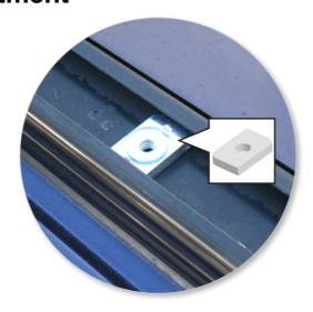
Slide metal T-nuts into tracks on vehicle.
