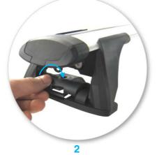
Select plastic internal block (from fitting kit) and insert it into foot
