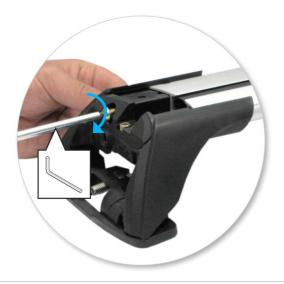
• Tighten adjusting screw to 5 Nm (3.7 ft lb).
