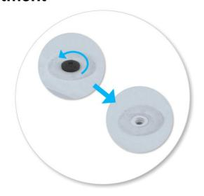
Remove fixed-point cover screws with 5mm (1/4") Hex Key.
