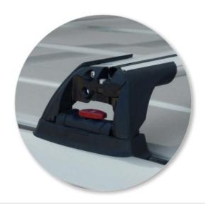
Ensure the red plastic knob is in the position shown when fully tightened.
