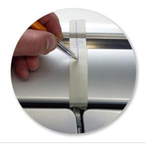
RECOMMENDED POSITION DUE TO AIRBAGS IN ROOF:
