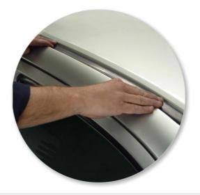
Re-install rubber ditch mould in roof channel.
