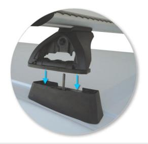
Place crossbars on pads ensuring the pads fit into the holes underneath the foot and the grubscrew pass through the hole in the foot.
