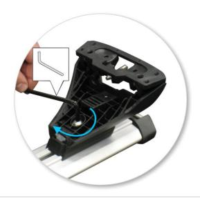
Using 5mm (1/4") Hex Key supplied with this kit, fully tighten to 5Nm (3.7 ft lb).
