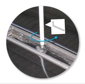
Remove screws from the vehicle's fixed points
