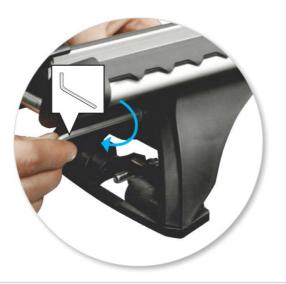
Once roof racks have been fitted to the vehicle, tighten adjusting screw to 5 Nm (3.7 ft lb).
