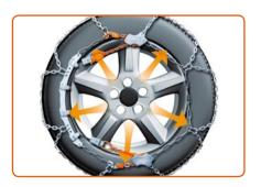
Please ensure that the chain mesh is lying evenly spread over the outer sidewall of the tyre.
