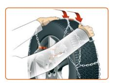
Slide the wire hoop over the tread until it lies on the back of the tyre. The back view on the right shows the wire hoop lying correctly on the inner sidewall of the tyre, which cannot be seen from the front.
