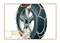
Now, on the lower part of the wheel, hook the grey hook (7) into the eyelet (8). Once again, this is easier if you pull the orange chain a little out of the ratchet. To do this, press the knob.
