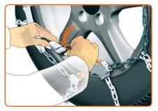
Now you just have to hook the two eyelets (9) into the plastic hook of the rubber tensioner (10).
