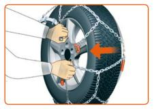
Grasp the chain mesh (11) near the orange hook and by the tensioning device. Pull it to the centre of the wheel. This brings the connector (3) to the front. Open the connector.
