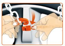
Now, on the upper part of the wheel, hook the orange hook (4) into the eyelet (5). This is easier if you pull the orange chain a little out of the ratchet (6). To do this, press the orange knob.
