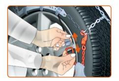
To remove the snow chains, park your vehicle so that the wheel comes to a halt with the orange hook (4) in the position shown in the diagram on the right. Then unhook the two eyelets (9) from the rubber tensioner (10).
