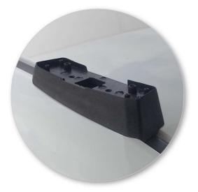
Place rubber pads (supplied with fitting kit) on the vehicle roof. Pad may vary in shape to that shown.
