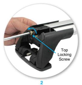
Use hex screwdriver supplied with crossbar to back off top locking screw for 10 turns.
