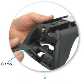
• Fit two front clamps (with holes) to one crossbar and rear clamps to another crossbar.
