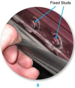
• Pull back door seal to gain access to fixed studs on vehicle body.
