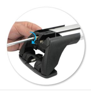
• Tighten adjusting screw to 5 Nm.
