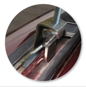
Locate clamp onto seam flange as shown (hook outboard, blade inboard). GB
