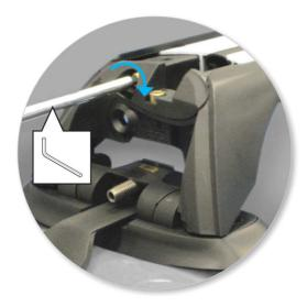
• Tighten adjusting screw to 5 Nm.
