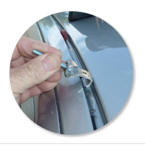
Hook clamps into the fixed point on the vehicle using inner slots.
