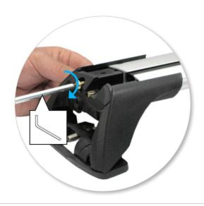
• Tighten adjusting screw to 5 Nm.
