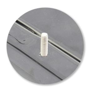
Install bolt with washer up through the fixedpoint from inside vehicle.
