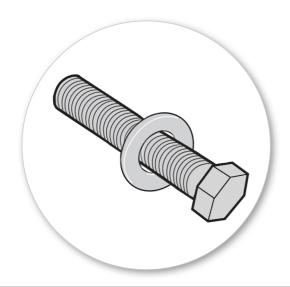
• Place flat washer onto 50mm bolt.
