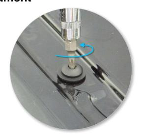
Remove rear screw only at each fixed-point position.
