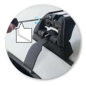
Tighten adjusting screw to 2 Nm (1.5 ft lb) hand tight.
