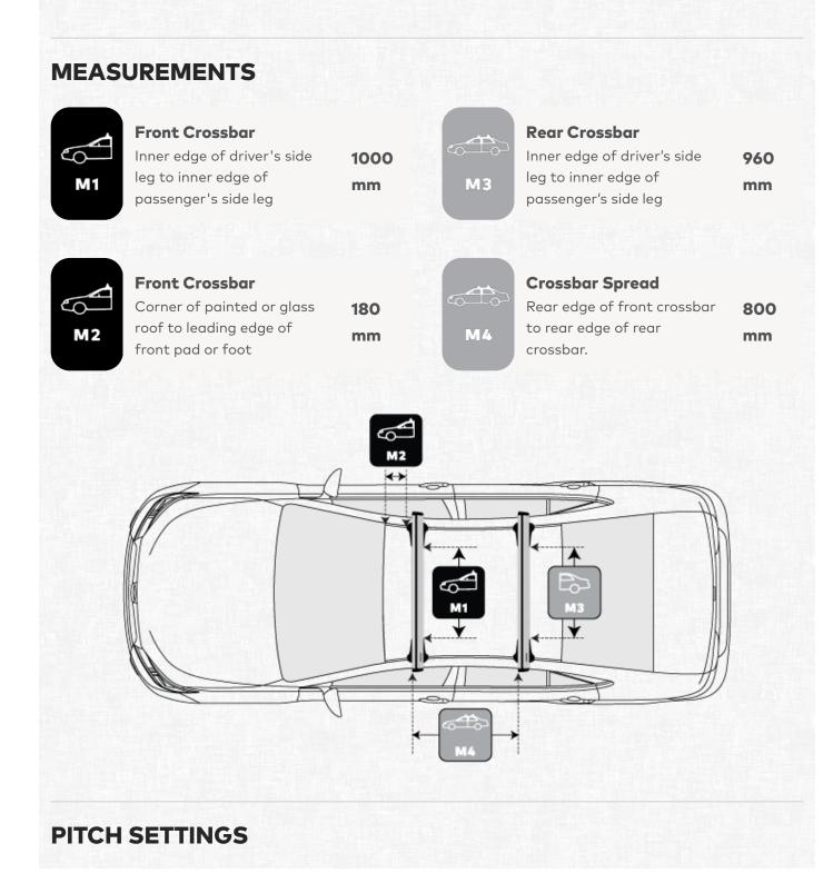
Pitch 1 Pitch 2  $\mathbb{D}$ Adjustment on the front Adjustment on the rear legs Α С legs to help keep the to help keep the crossbars Ρ2 Ρ1 crossbars level level 6° œ P
